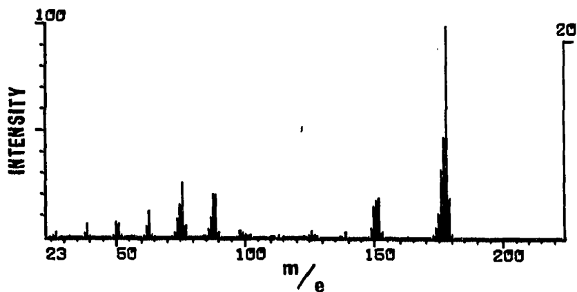
Fig. 6. Mass spectrum of GC effluent peak No. 149 of coal tar volatile sample.
